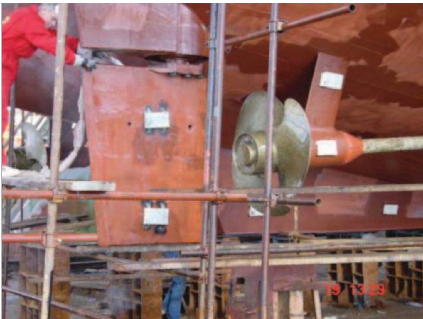
Figure 3. Protection of the rudder blade with VpCI®
