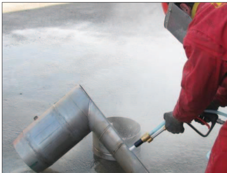
Figure 10. Surface preparation with wet blasting process
