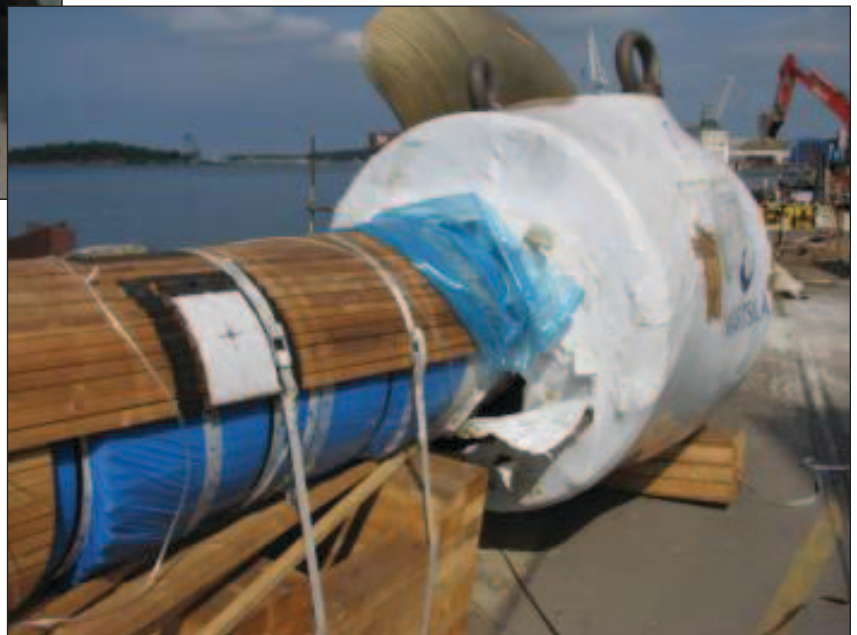
Figure 8.b Protection of equipment with VpCI® 126 film
