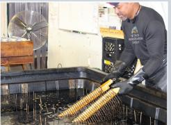
MPG uses an all chemical process. No abrasives are ever used, thereby protecting microfinishes and tolerances.
