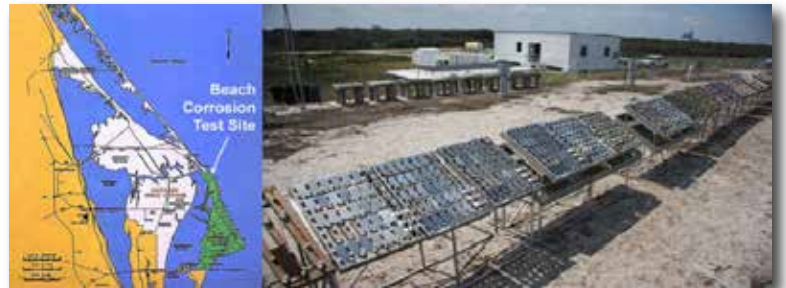
Location of the beachside corrosion test site at Kennedy Space Center, Florida, along the Atlantic Ocean (left) and panels after initial CPC application and exposure to the marine atmosphere at the test site (right).
