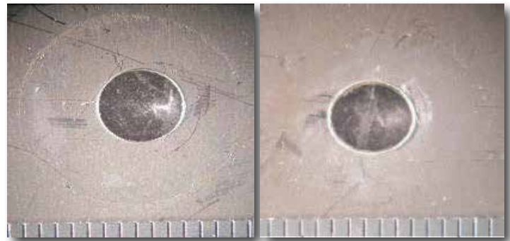
Examples of crevice corrosion for atmospheric exposure of CPC-coated stainless steel (left -control and right - Cortec's EcoLine 3690)
